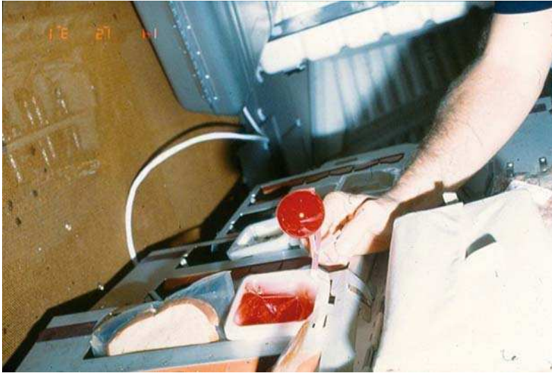
FIGURE 9.3 The STS-5 crew demonstrates what happens when straw is not clamped shut on the rigid beverage container (NASA photograph).
